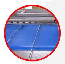
Synthetic egg belt and hand packing table with adjustable dividing lanes for all grades of seven weights
