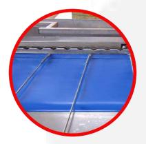
Synthetic egg belt and hand packing table with adjustable dividing lanes for all grades of six weights
