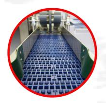
In line feeding conveyor with special modular chain belt made in food plastic material. Innovative and easy to clean.
