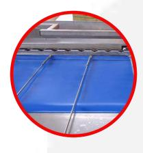
Synthetic egg belt and hand packing table with adjustable dividing lanes for all grades of seven weights
