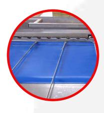
Synthetic egg belt and hand packing table with adjustable dividing lanes for all grades of seven weights
