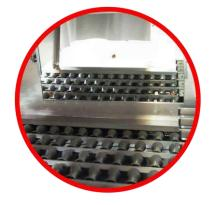
All Riva Selegg egg graders are equipped, as standard, of a section dedicated for candling eggs with lamps. On demand are available different types of lamps
